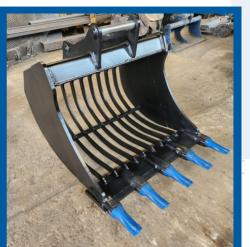
The customer manufactured a 1200mm wide clamshell bucket in Hardox. The bucket is multipurpose for an 18-tonne machine. He chose to place his trust us by installing 5 TURNKEY® Grizzly kits with a standard tooth shape.
