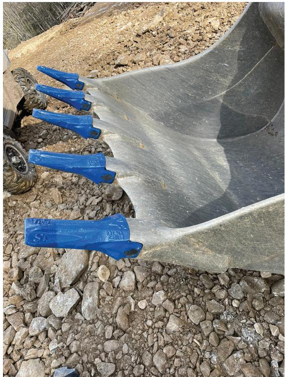
*TURNKEY® Grizzly a new line of ground engaging tools using hammerless locking devices with permanent compression for teeth.*
