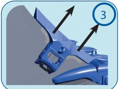
Shroud removal: Once the pin is removed, you can easily remove the shroud
