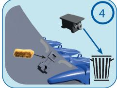
Shroud adapter cleaning: Clean up the shroud adapter and the pin housing.
