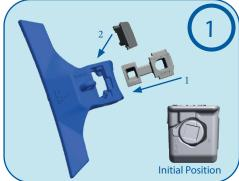
Pre-Assembling: Pre-assemble the 3 parts: Adapter, shroud and pin.
