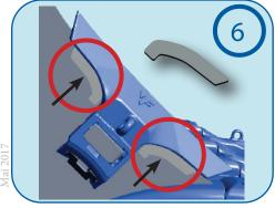
Instruction de soudure (étape 3): After having installed and locked the pin, we will recommend welding shroud supports, just to absorb the forces on the wing.
