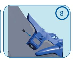
Protective caps installation: On both shrouds sides, insert the protective caps to avoid fines to fill up the pin hole.
