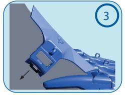
Adapter shroud positioning: Raise the bucket to an angle of approximately 30°. Position the shroud assembly on the Wing. Position adapter on wing, once the adapter is correctly located.
