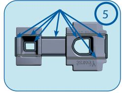
Welding instructions (step 2): Once shroud adapter has been properly oriented and fixed by welding spots, remove pin and shroud. Heat the adapter at 175°-200°C and weld the areas indicated above.
