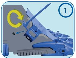
Pin unlocking: Remove the protective cap and insert the TK OD® tool into the pin, unlock the pin with a 180° clockwise turn.
