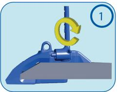
Pin unlocking : Remove the protective cap and insert the TK OD $\circledast$  tool into the pin, unlock the pin with a 180° clockwise turn.
