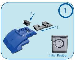
Pre-Assembling : Pre-assemble the 3 parts : Adapter, shroud and pin.
