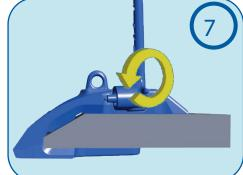
Pin clamping : : Re-assemble the shroud and pin on the adapter
