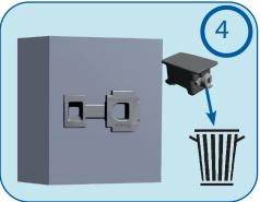
Shroud adapter cleaning : Clean up the shroud adapter and the pin housing.
