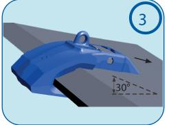
Adapter shroud positioning: Raise the blade edge to an angle of approximately 30°. Position the shroud assembly on the bade.Pull the adapter toward the center. Position adapter on blade, once the adapter is correctly located.
